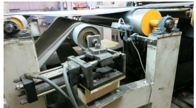
Conveyor Guider (Hydraulic) is used on a Floor Tiles Machine
